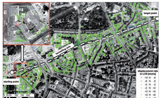
Figure 3: Aerial map of the eastern branch of the Wehrhahn-Linie in the state capital city of North-Rhine Westfalia Düsseldorf, Germany with displacement-rates in LOS (mm/year), acc. to [6]
