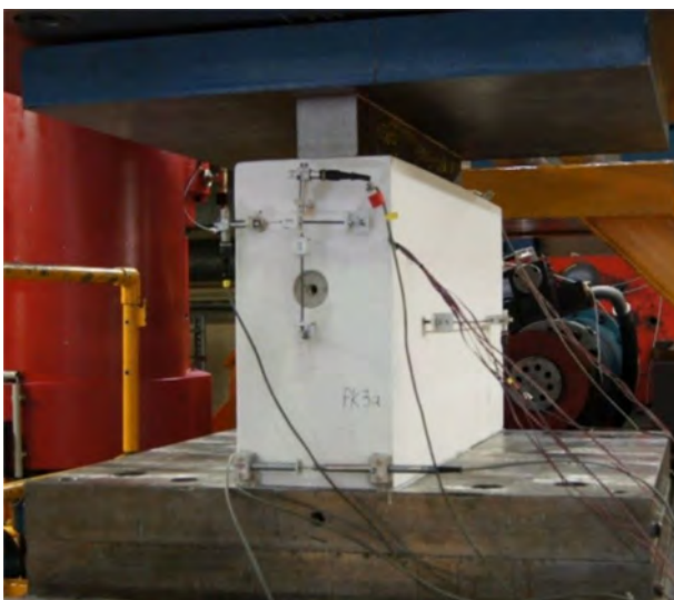
FIGURE 3 Basic experimental setup of series A with introduction of partial area strip loading
